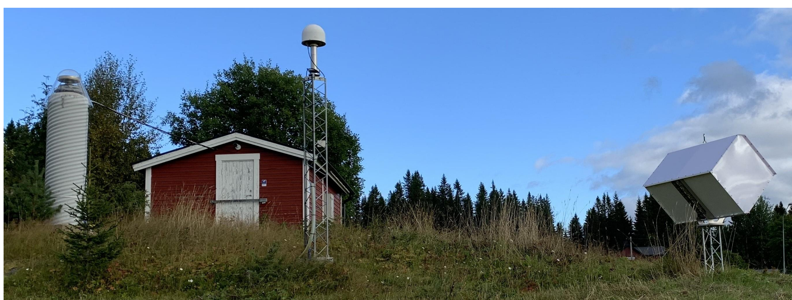
Figure 1: SAR reflectors have been installed co-located with the 21 fundamental SWEPOS stations, both passive reflectors (corner reflectors) and transponders.
