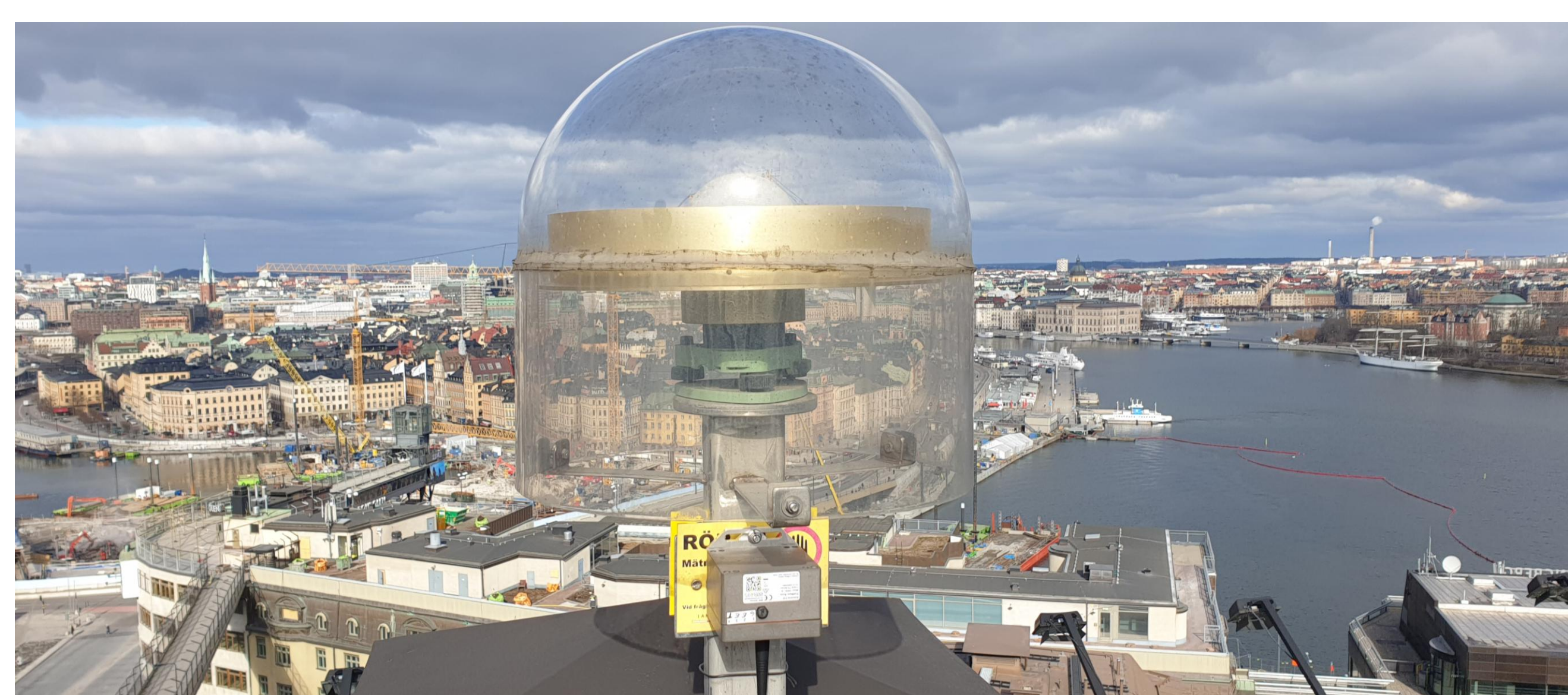
Figure 3: Using inclinometer for stability monitoring of GNSS continuously operating reference station.
