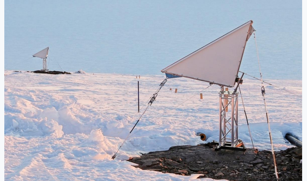
Triangular trihedral CRs in Aboa Research Station, Antarctica
