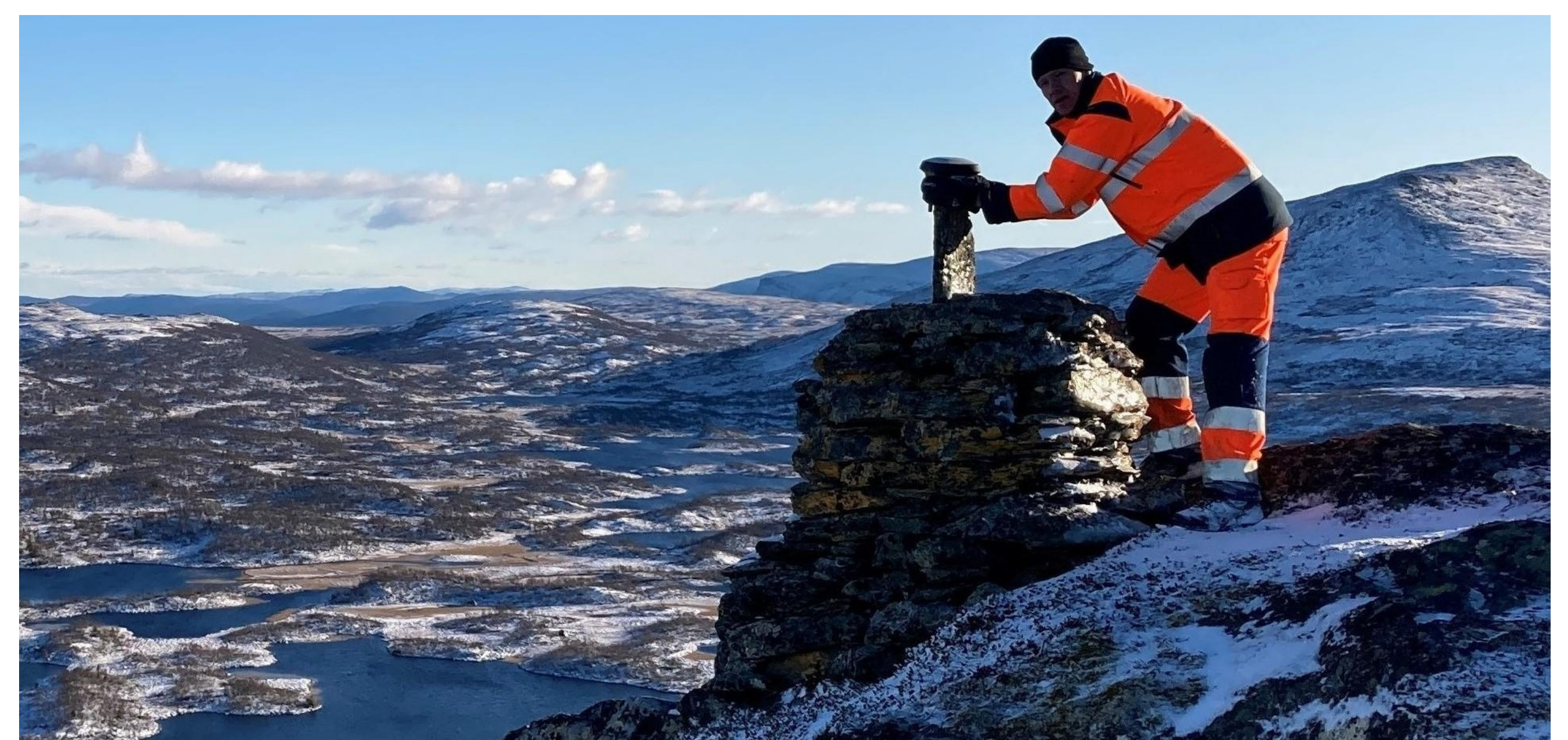
Figure 4: All boundary markers were surveyed with GNSS (mainly network RTK through SWEPOS or CPOS services). This boundary marker is a so-called utliggare.
