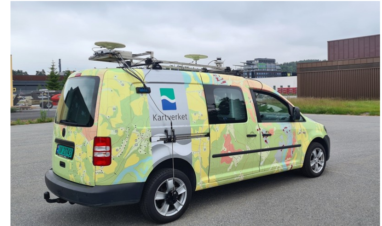
Figure 1. The Norwegian Mapping Authority's Measuring Car with navigation system: GNSS, IMU, Odometer and LiDAR.
