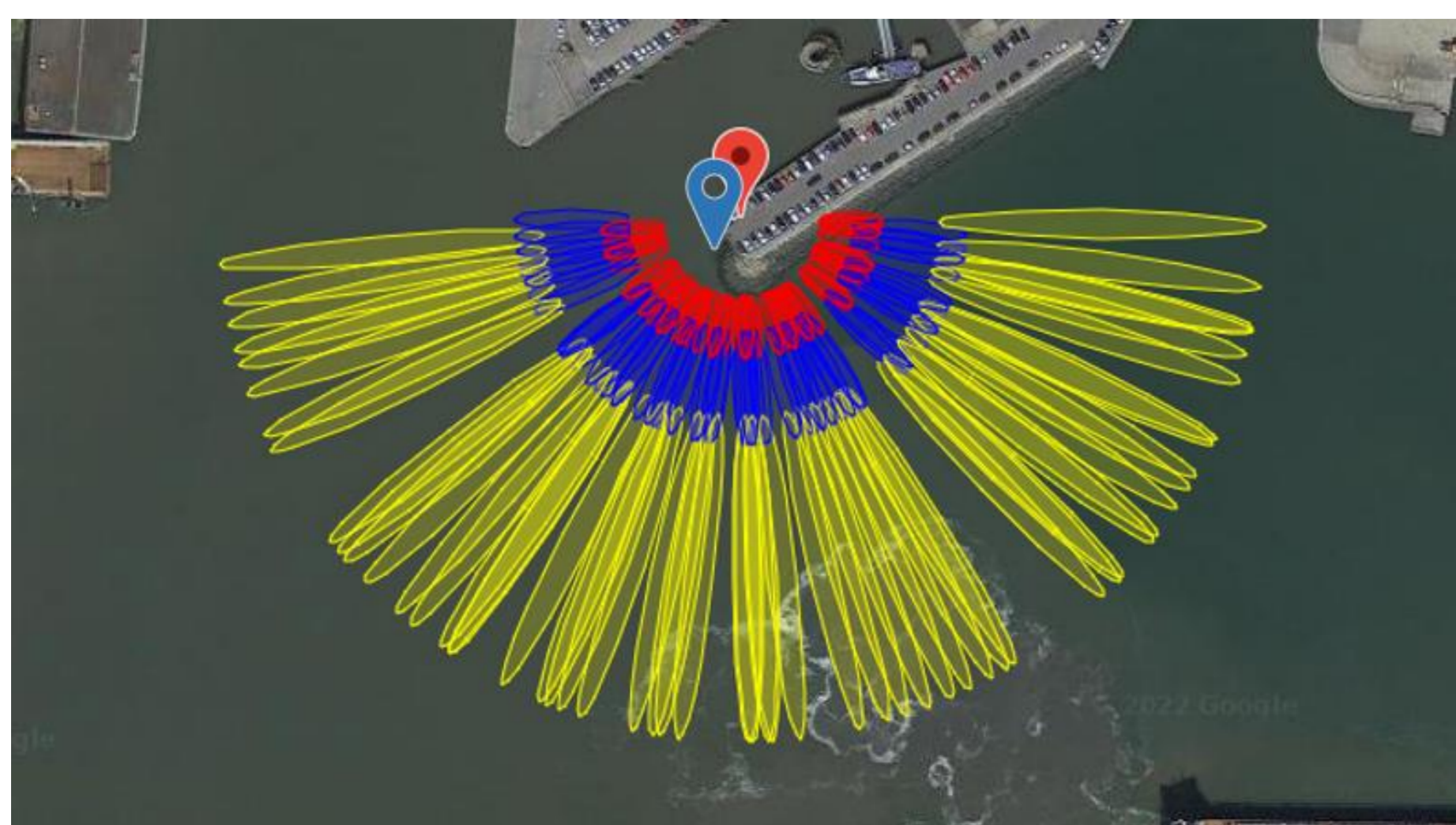
Fresnel zones at Esbjerg Harbour. GNSS station marked with a red arrow and tide gauge marked with a blue arrow.
