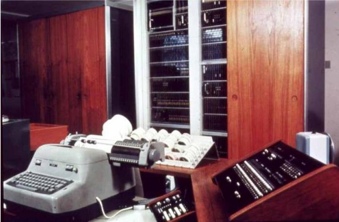
The Geodetic Software System, originating at the Danish Geodetic Institute, was based on ideas from the 1950s, and found its first true incarnation in the Algol language and the custom built geodetic number cruncher GIER (figure left), from 1961.
