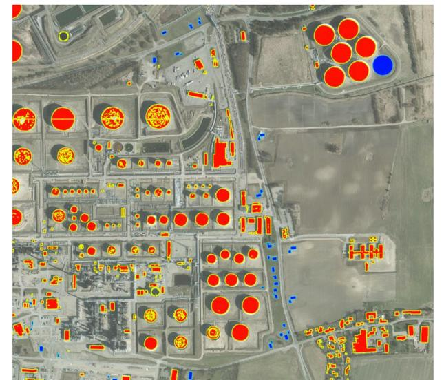
When combining existing map data with new LiDAR data, synergistic potentials show up.
