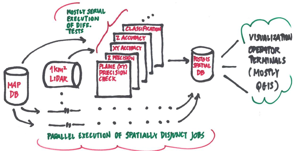
**Above:** The QC system works on individual  $1 \text{ km}^2$  square tiles in parallel. The results are collected in a spatial database.
