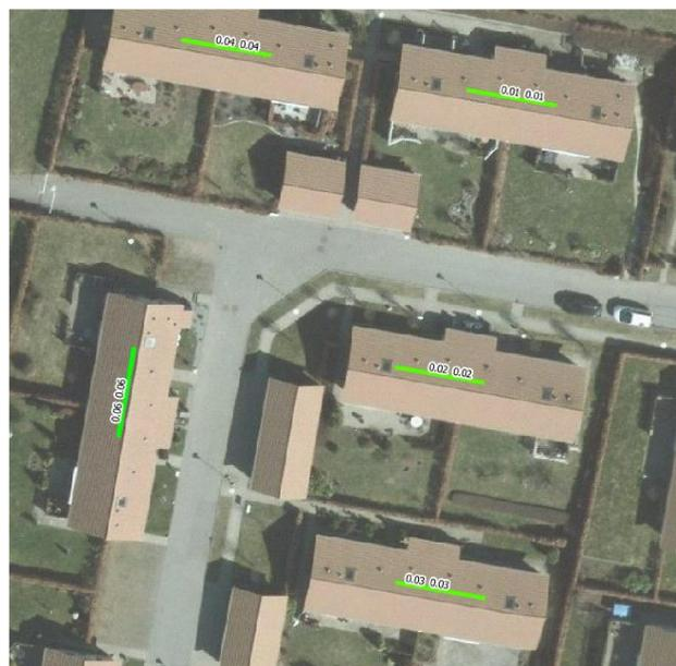
**Above:** Plane precision by dual ridge detections. The offsets observed with respect to the orthophoto background are as expected, since the orthophoto processing is based on a terrain model, which does not include the building heights.
