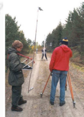
Figure 14: Adjustment of Wild N3 in 1996. The record keeper notes the red readings on a HandyThermo computer. As a part of the table there are temperature sensors 0.5 and 2.5 m above the ground.
