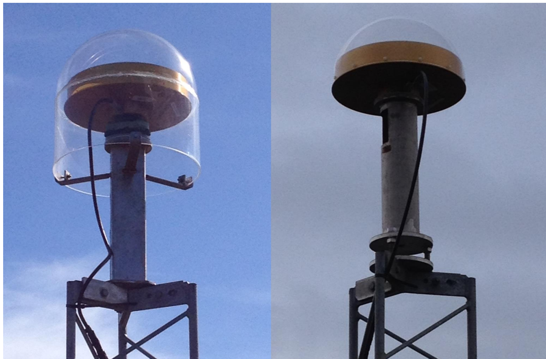
Figure 1: The OSOD radome to the left and the OSOS radome to the right. Photo: Johan Löfgren, Onsala Space Observatory, April 2015.
