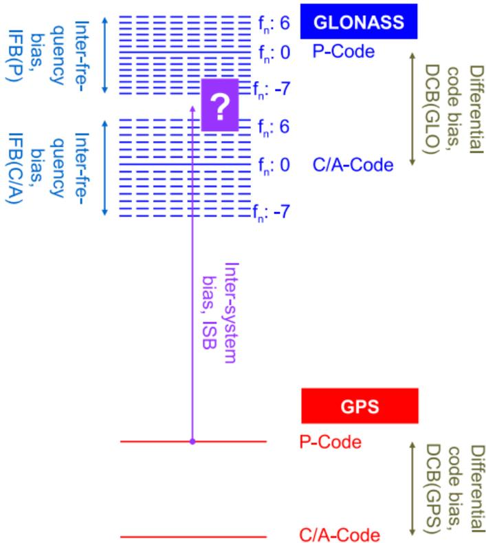
We can only extract the sum of delays from a GPS/GLONASS data processing.
