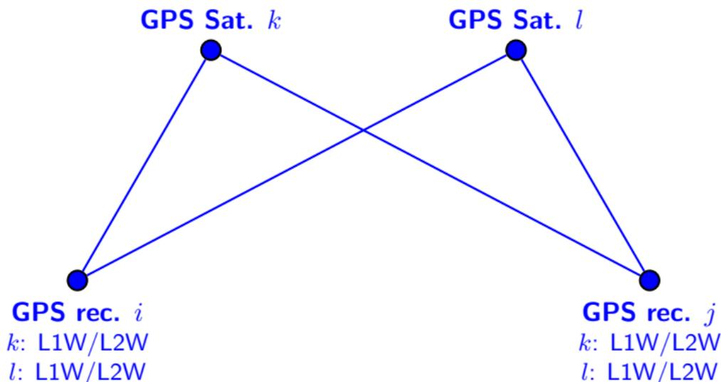
$$\begin{array}{ll} k: \alpha_i(L1W) & \alpha_i(L2W) \\ l: \alpha_i(L1W) & \alpha_i(L2W) \end{array}$$
