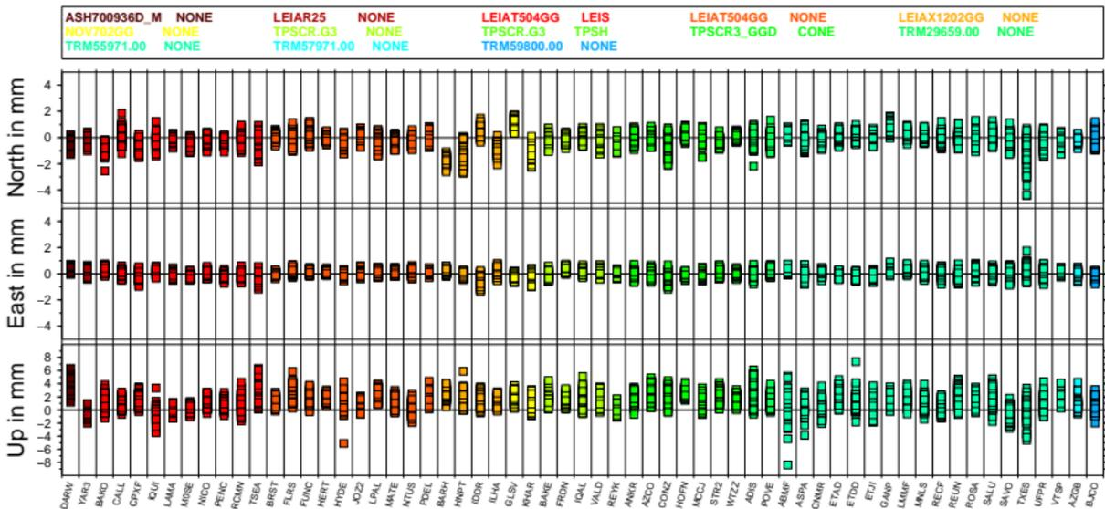
GPS–GLONASS–Bias for the coordinates using IGS05.atx–antenna phase center corrections from weekly solutions of the years 2009 and 2010.
