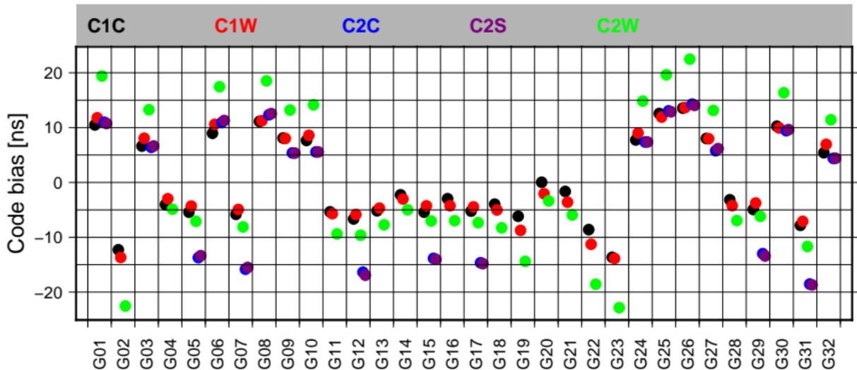
Bias solution for GPS satellites based only on CLK+ION: [reference C1W](#)
