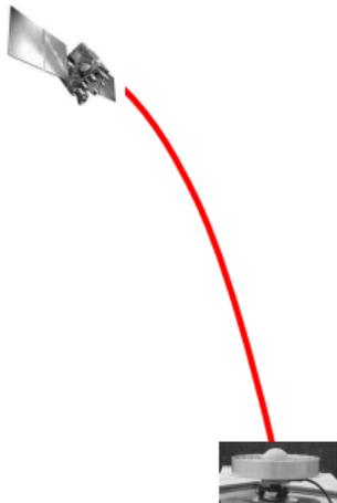
$I_i^k$  signal delay in the ionosphere
