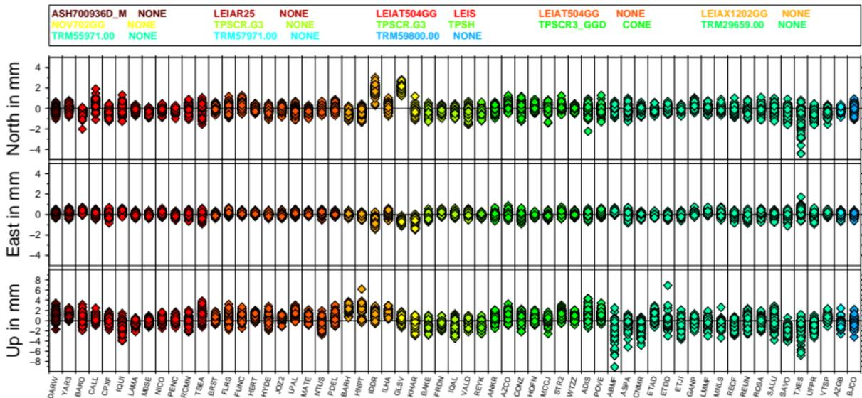
GPS–GLONASS–Bias for the coordinates using IGS08.atx–antenna phase center corrections from weekly solutions of the years 2009 and 2010.
