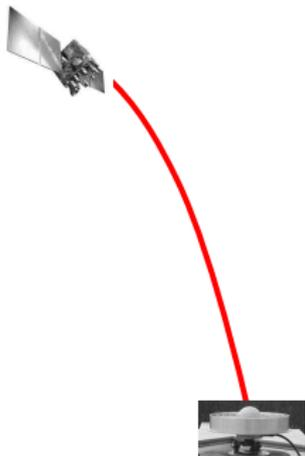
$I_i^k$  signal delay in the ionosphere
