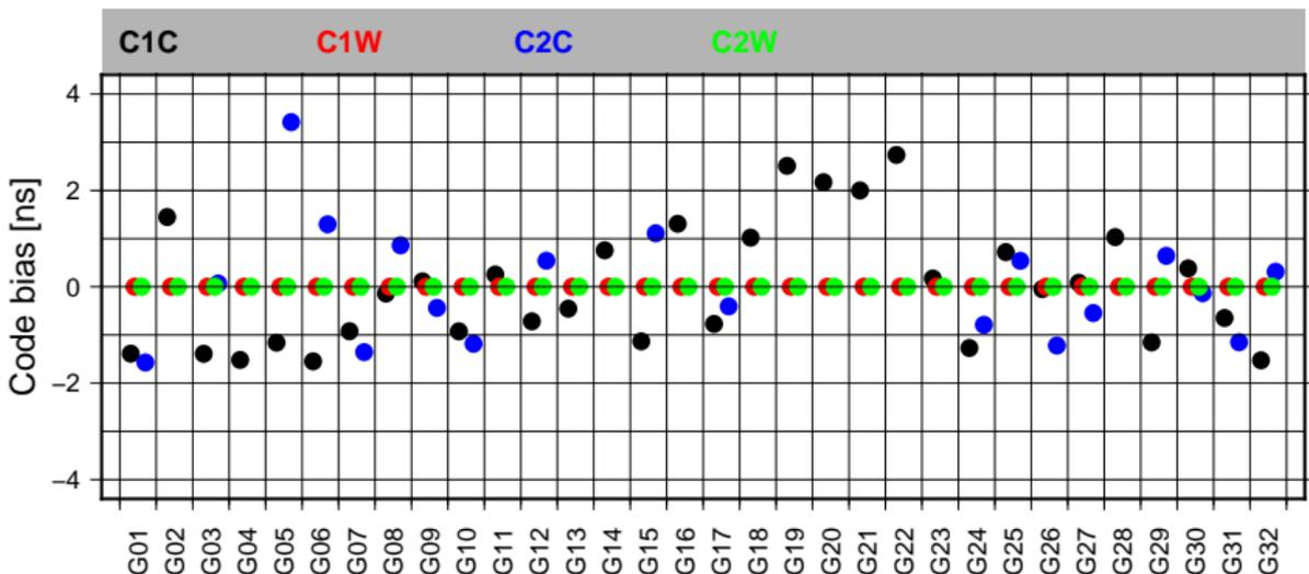
Bias solution for GPS satellites based only on CLK:
