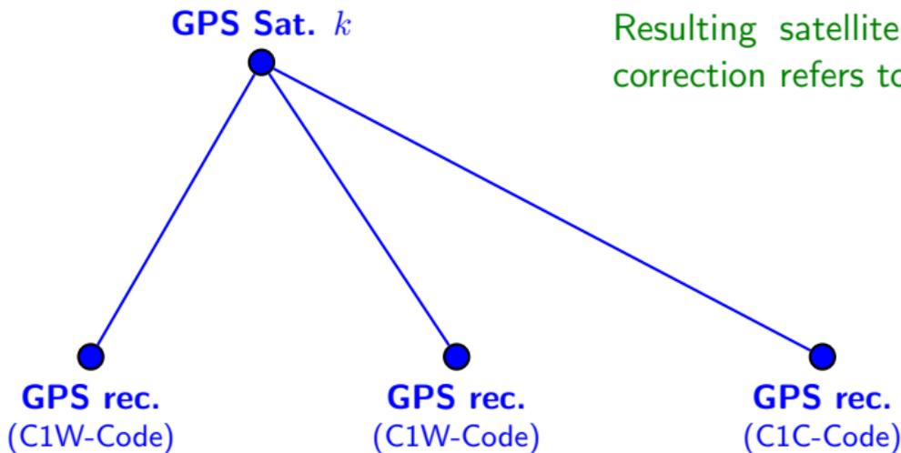
$$\begin{aligned} & \text{GPS-sat clock} \\ & \delta^k + a^k(C1C) \\ & + DCB^k(C1C - C1W) \end{aligned}$$
