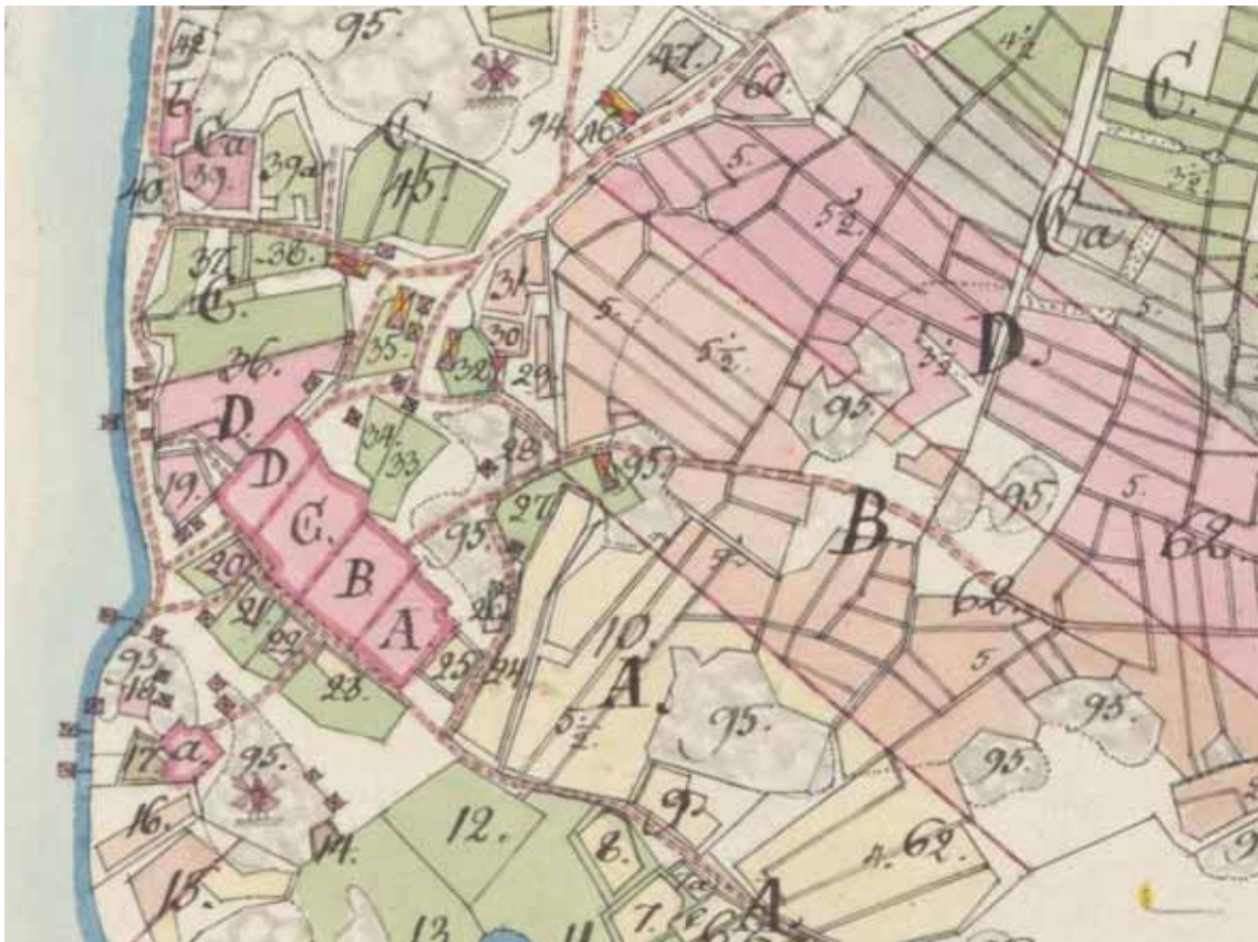
Figure 2. The newer maps especially from the 18 th century and onwards are usually based on measurements and can be very accurate. A detail from an enclosure map from Ilavainen, Eurajoki, Finland, from 1813 scanned with a flatbed scanner at the resolution of 300 ppi by the National Archives of Finland.
