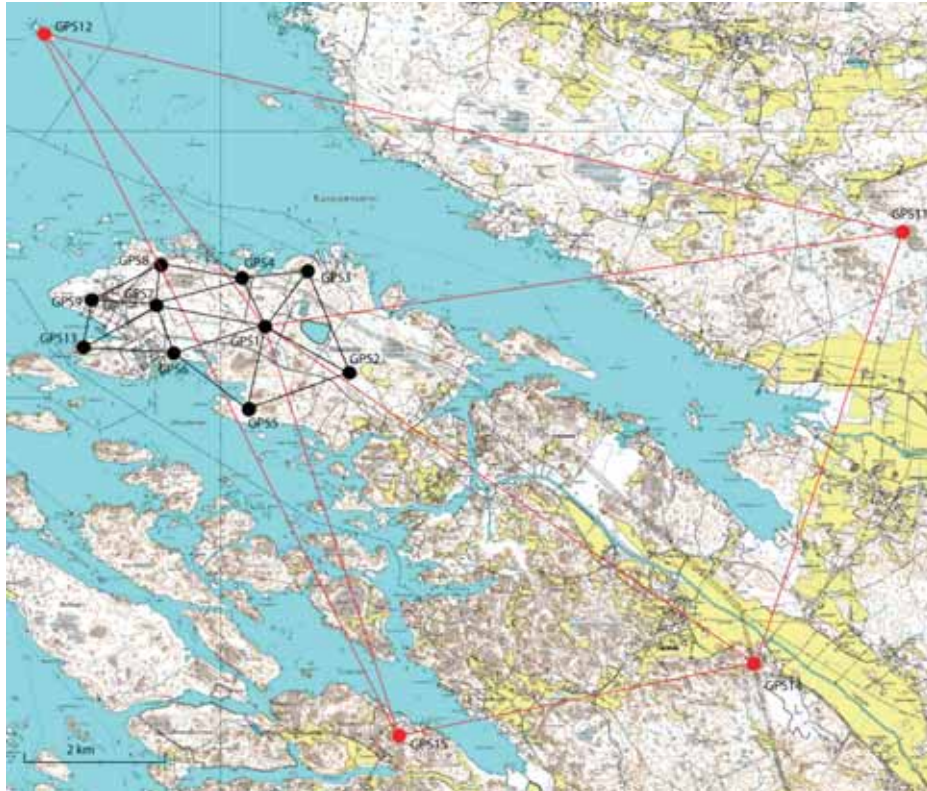
Figure 1. The GPS networks of the Olkiluoto. The main network on Olkiluoto Island has been observed twice a year since 1995. The surrounding network has been established in 2003-2005.
