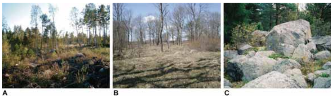
Figure 4. Different types of till in the Forsmark area. A) Sandy till with a normal frequency of boulders, B) Clayey till with a low frequency of boulders, C) Till with a high frequency of large boulders.
