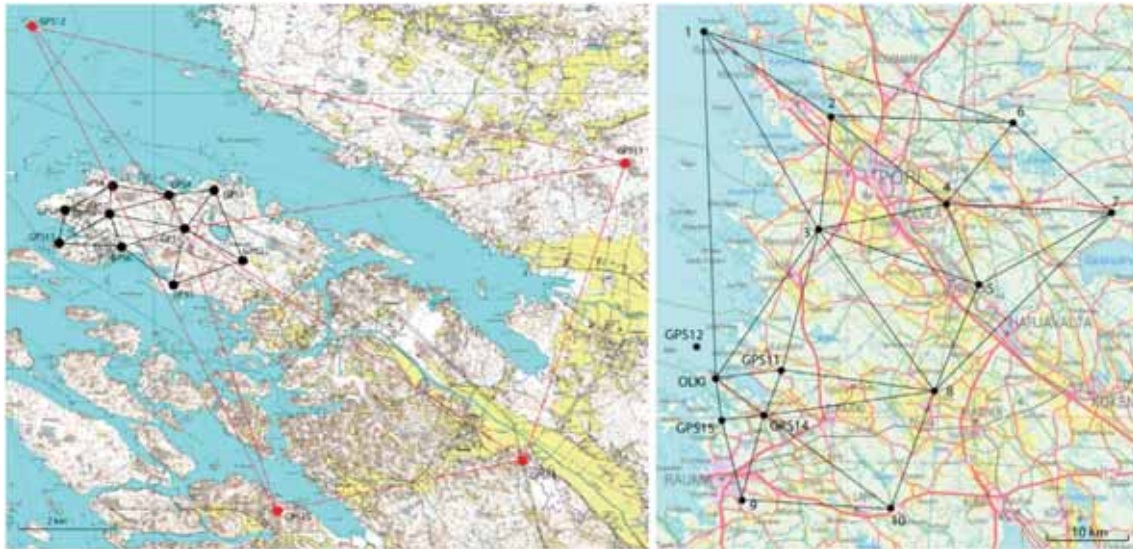
Figure 5. (Left): The local GPS monitoring networks at the investigation area of Olkiluoto. Black: Original network has been established in 1994 (GPS13 in 2003). Red: Pillars have been established in 2003 and 2005. (Right): GeoSatakunta GPS network. Base map ©National Land Survey, license number 51/MML/09.
