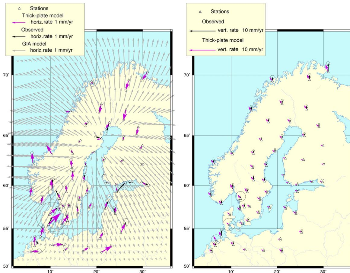
Fig. 4. Residual motion (GPS minus GIA model), horizontal velocities left, vertical right, and the thick-plate solution.
