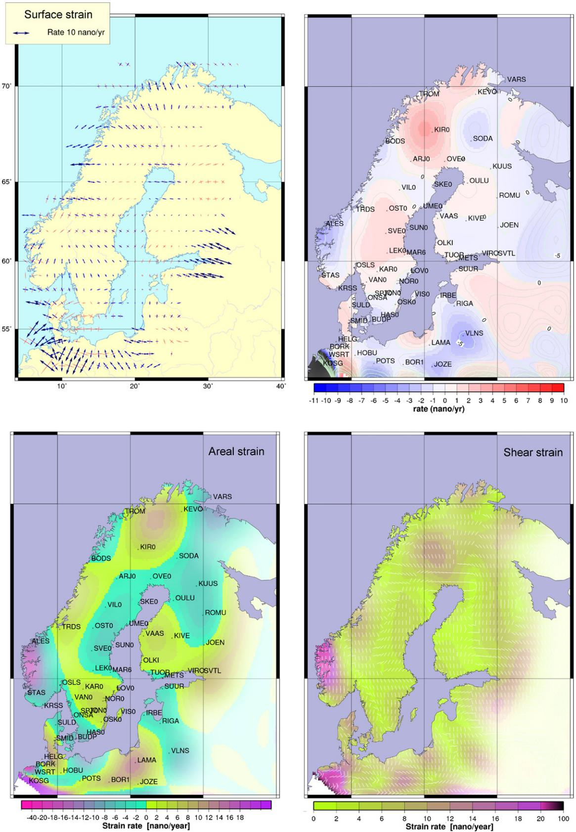
Fig. 5. Thick-plate solution for surface strain rates (left) and curl (right) derived from the residual observed motion after subtracting the GIA predictions.
