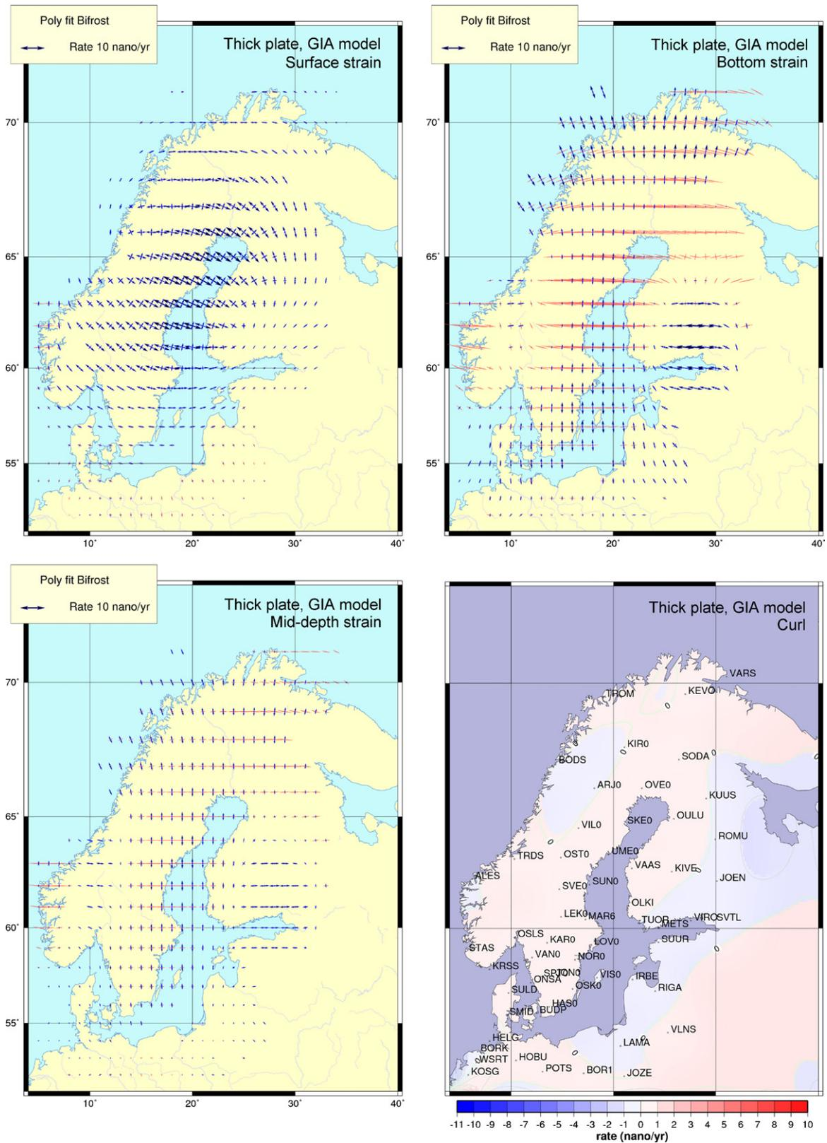
**Fig. 3.** Strain rates computed by the thick-plate model at surface and bottom of the slab (top row) and at mid-plane depth (bottom left). Curl is shown in the bottom right map.
