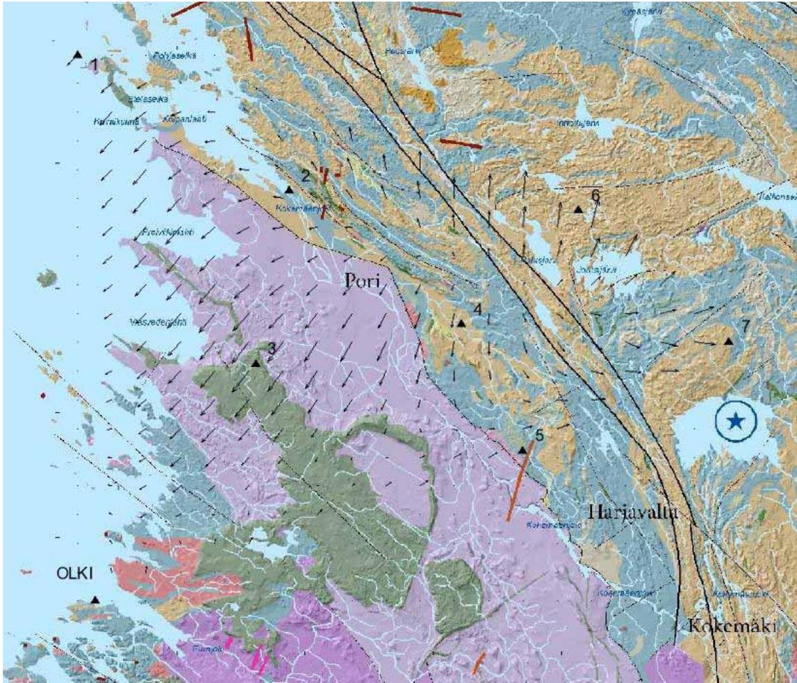
**Figure 6-9.** The estimated velocity vectors are slightly diverging in the vicinity of geologically interesting features, like the major shear zones (black solid lines) and Jotnian sandstone (see legend of Figure 1-1). Base map © Geological Survey of Finland.
