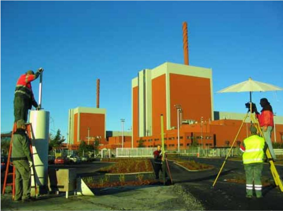
*Figure 2-7. Precise levelling at Olkiluoto. (Photograph J. Ahola.)*
