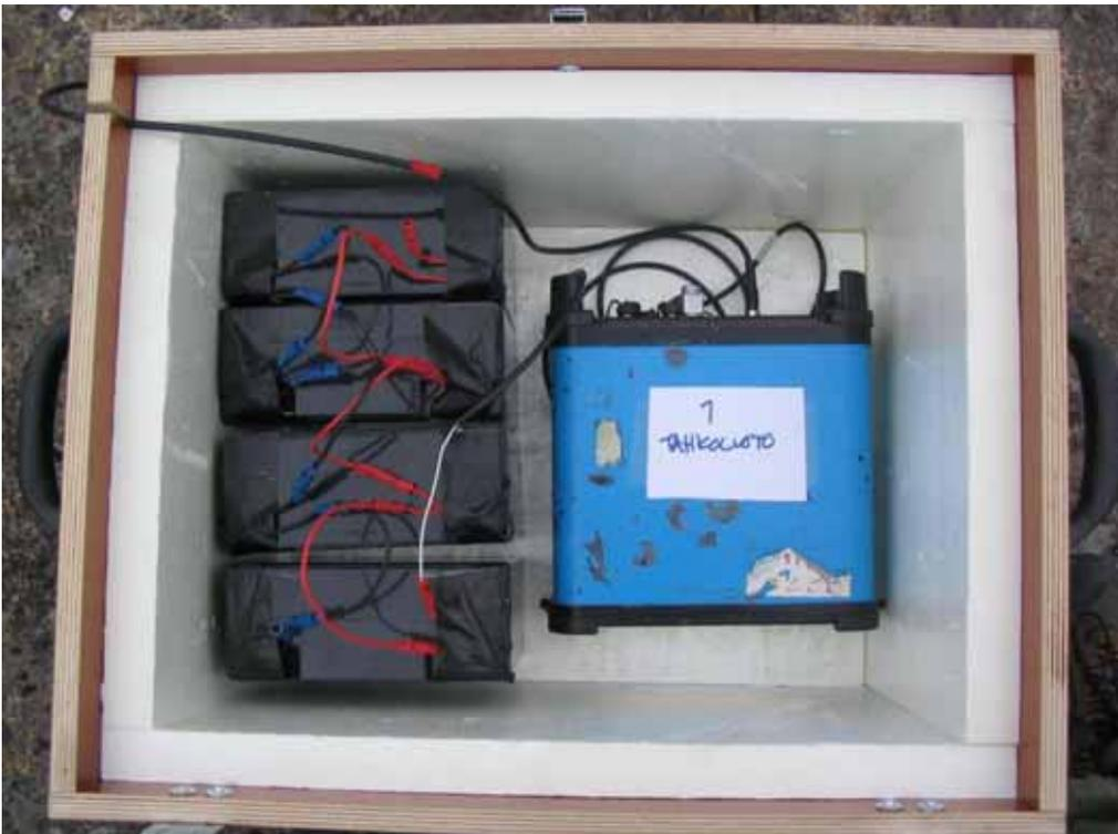
*Figure 4-6. Receiver and batteries in the instrument box. (Photograph J. Ahola.)*
