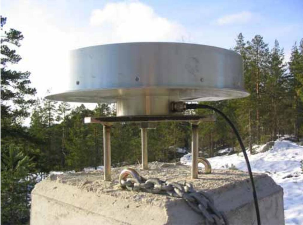
*Figure 4-5. A Dorne Margolin type antenna on a pillar. (Photograph J. Ahola.)*
