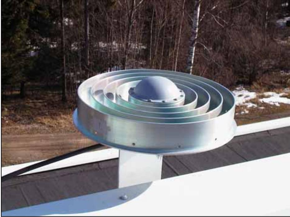
**Figure 3-3.** Dorne Margolin type choke ring antenna. This kind of structure damps the effect of multipath. The antenna type is a de facto standard in precise GPS measurements. (Photograph M. Poutanen)
