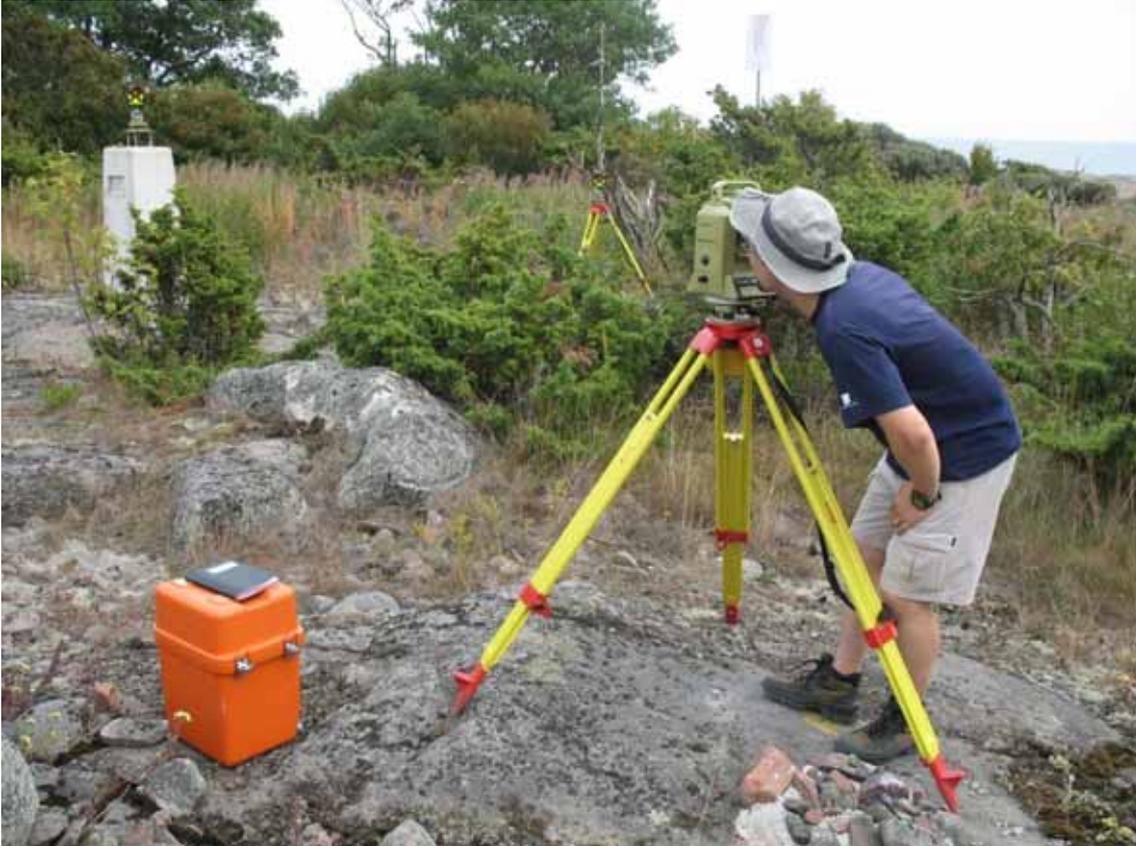
*Figure 4-9. Centering measurement of the pillar at Tahkoluoto. (Photograph J. Ahola)*
