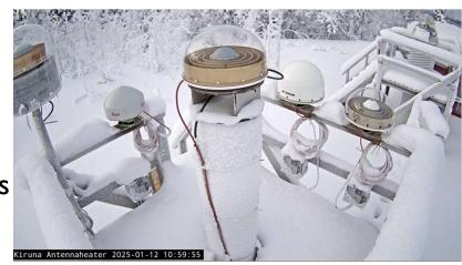
Tests on a Swepos concrete pillar, we see that we need some more heat to make the snow melt away also on the lower part of the radome as the radome is bigger. The GNSS antenna to the left in the picture does not have a heated choke-ring.
