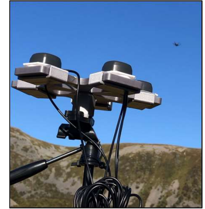
2nd array: circular, patch antennas (UCA: Uniform Circular Array)
