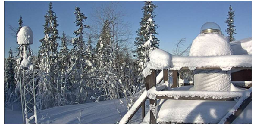
Wide-brimmed OSOD radome to the right.
