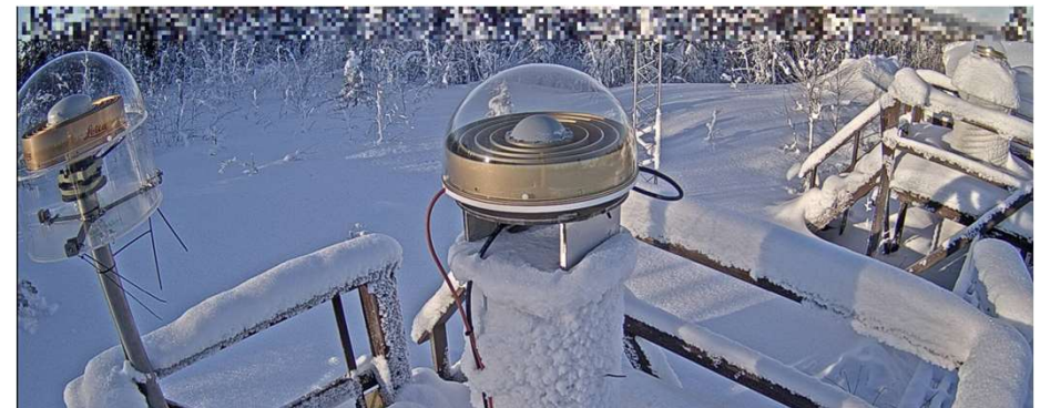
OSOD radome with bottom plate to the left, OSOS radome to the right.
