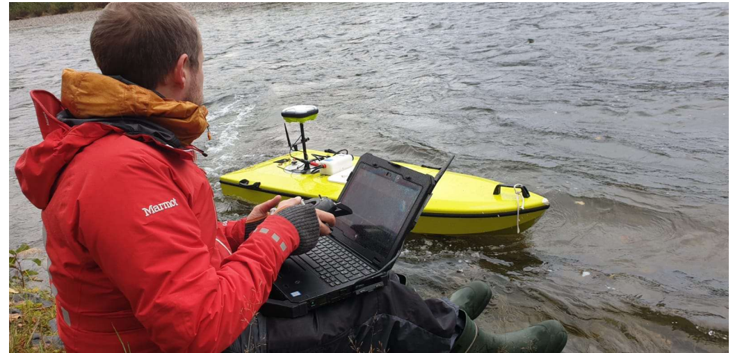
NVE uses CPOS for bathymetric mapping. Photo: Line Dale, NVE.
