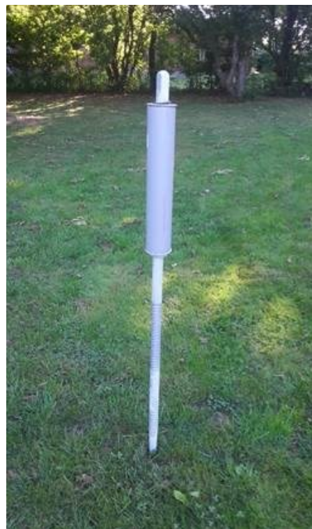
Figure 5 The 1.5 m long torsional plug ready to be mounted into the ground.
