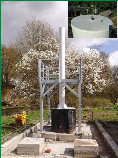
Prototype of the geodetic support point, suitable for long-term observations
