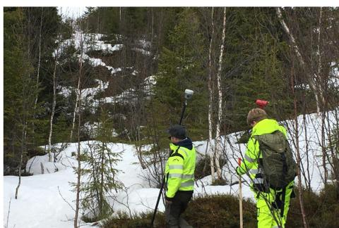
**Figure 10:** To be able to get a straight five-metre-wide clearing between the boundary markers, the boundary line is set out with network RTK and marked with wooden sticks. Picture: Dan Norin.
