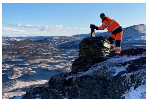
**Figure 11:** “Utliggare” are smaller stone cairns which only show the boundary line, not defining it. These are also measured with GNSS. Picture: Karl Tirén.
