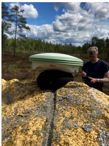
**Figure 5:** Norwegian Boundary Commissioner Anders Østeraas is surveying Rr 52B with a network RTK service (SWEPOS or CPOS). Rr 52B consists of a large natural stone. Picture: Dan Norin.
