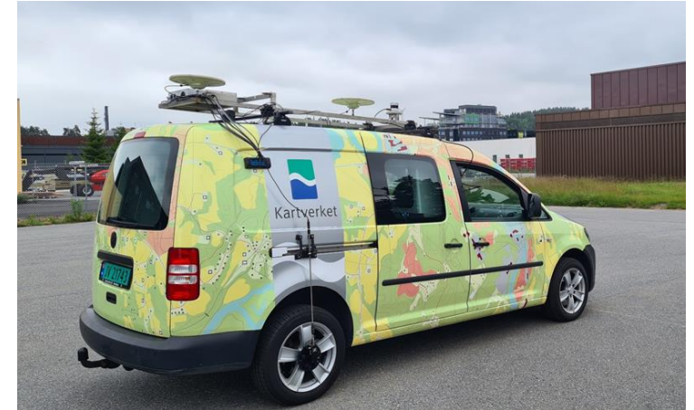
Figure 1. The Norwegian Mapping Authority's Measuring Car with navigation system: GNSS, IMU, Odometer and LiDAR.
