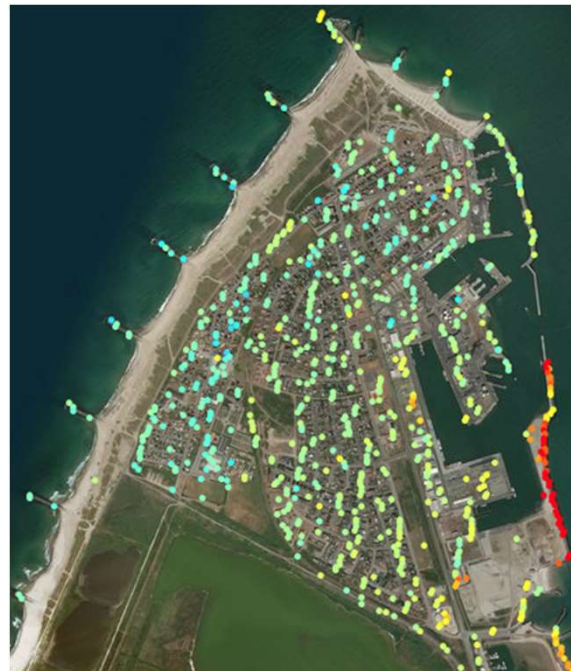
Subsidence (single track: 139D)
