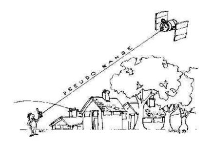
Satellite coordinates and clock corrections (x<sup>s</sup>,y<sup>s</sup>,z<sup>s</sup>,dt<sup>s</sup>) are received from satellites
