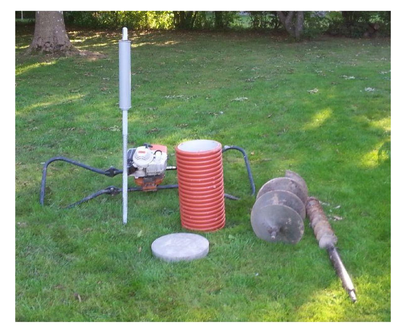
The installation tool kit for torsional plugs is shown to the right - it includes a light weight, but powerful petrol powered auger. The plug is shown with the grease filled casing mounted. The well pipe and well cover is installed before the plug is screwed into the lower parts of the topsoil.
