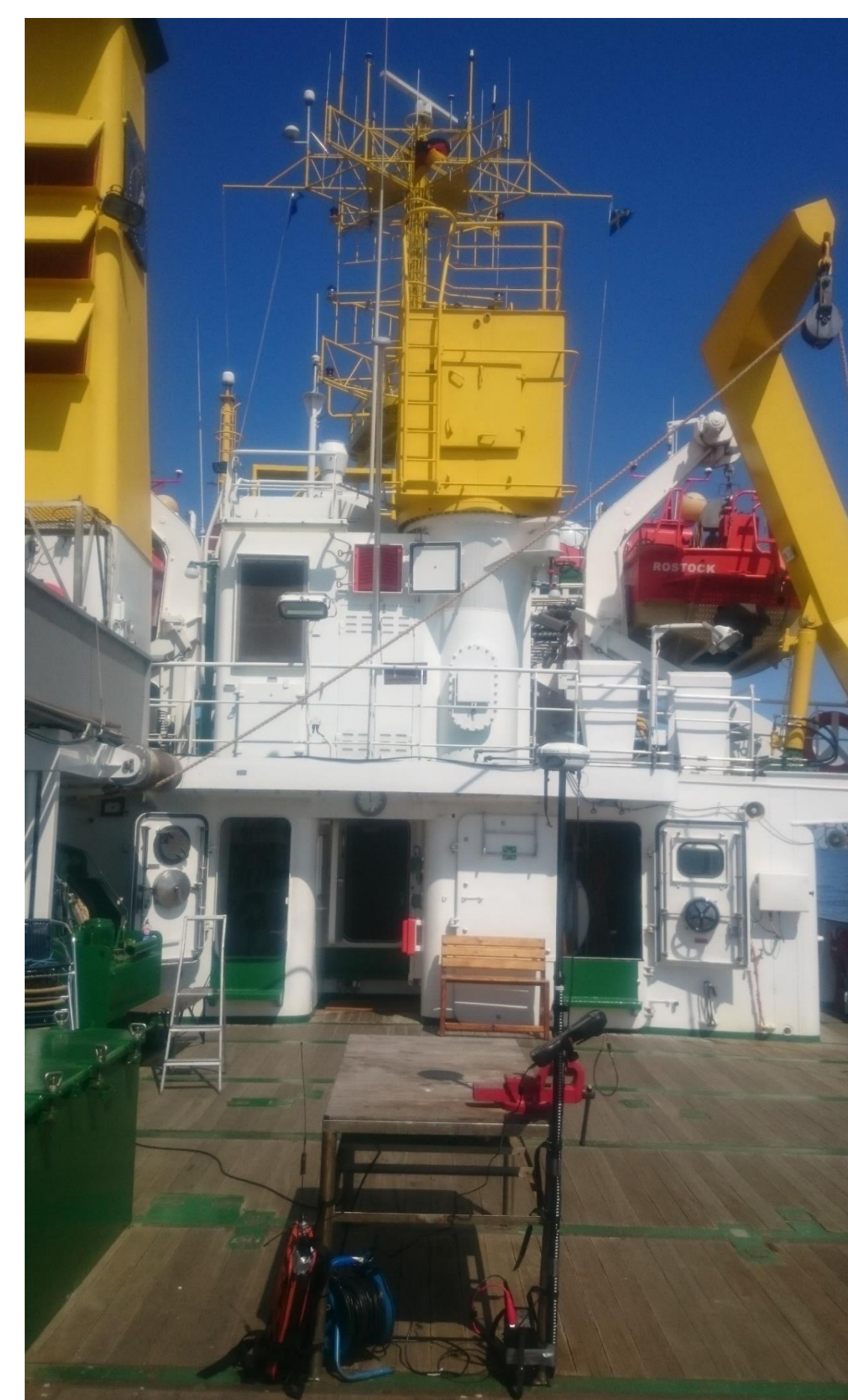
Figure 2: The RTK rover mounted on the stern deck of the vessel. The external GNSS antenna for the other test is mounted on the mast of the vessel. Photo Kent Ohlsson.
