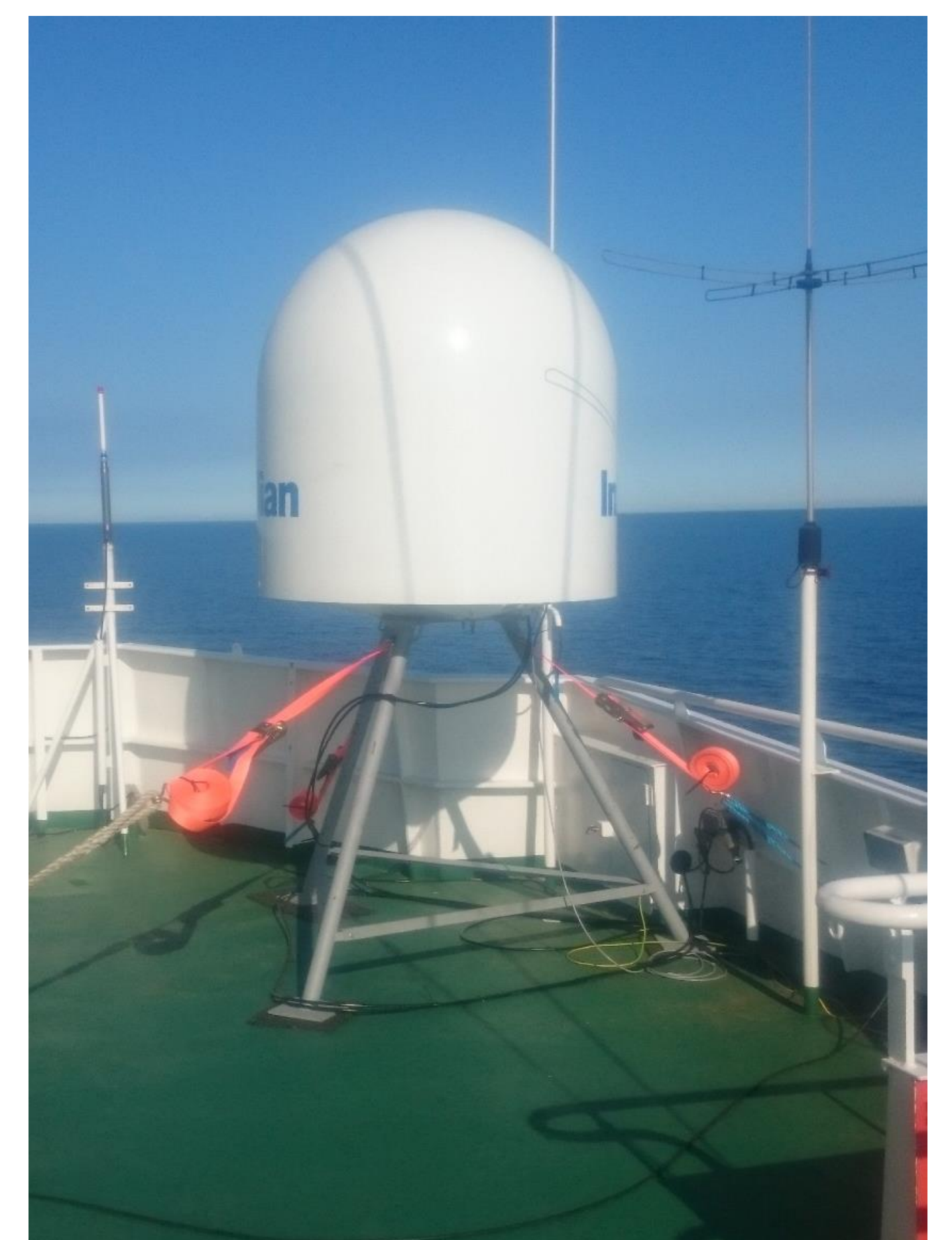
Figure 3: One of the two antennas used for the communication with the reference network through a VSAT satellite link. Photo: Kent Ohlsson.
