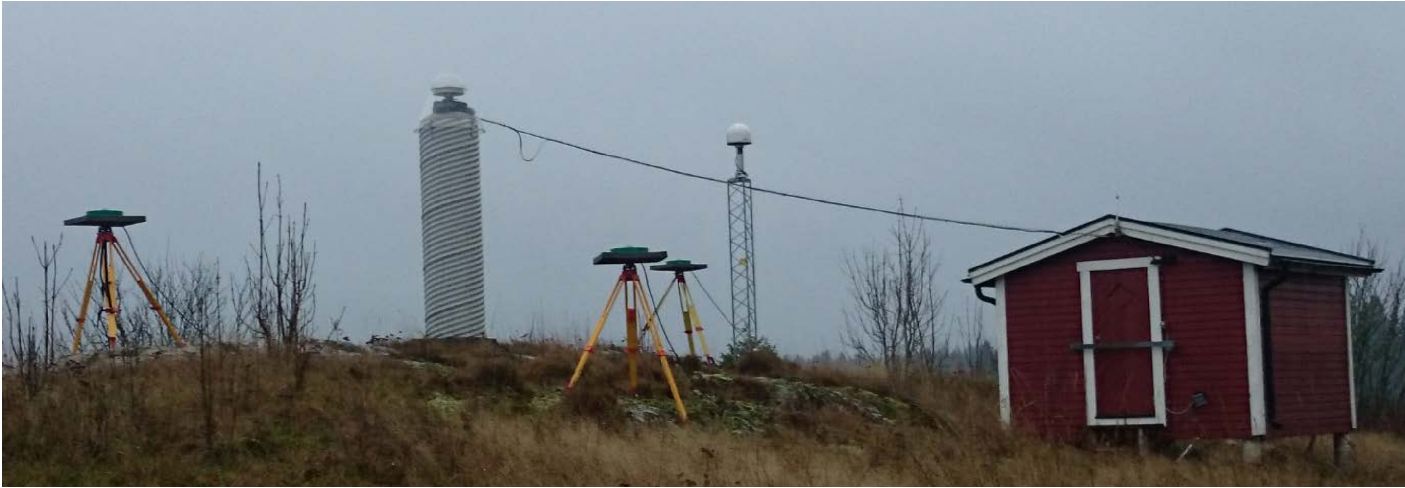
Figure 1: Station calibration at the SWEPOS site Vänersborg. Photo: Kent Ohlsson, 2015.
