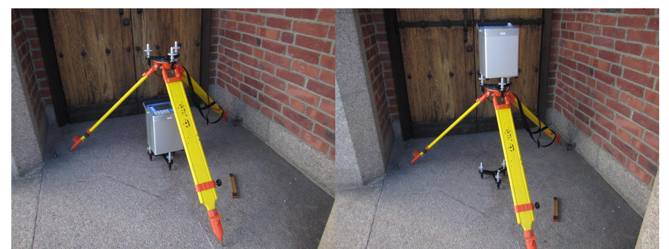
Gradient measurements for an A10-site, Östersund RG62. The instrument used is a Scintrex CG5. The idea is that the height difference between the set-ups should be as close as possible to the sensor height of A-10, which is 70 cm.
