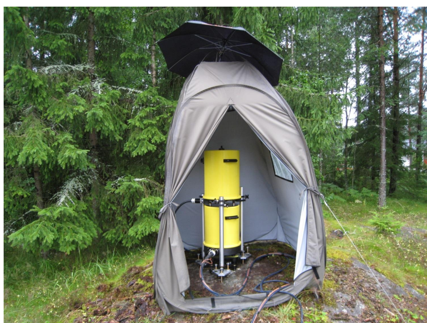
A-10 measurements, at Säffle (first order RG82-site) in rain. The tent shall protect the A-10 from sun, wind and rain. This tent was though broken at the top, thus an umbrella was needed.
