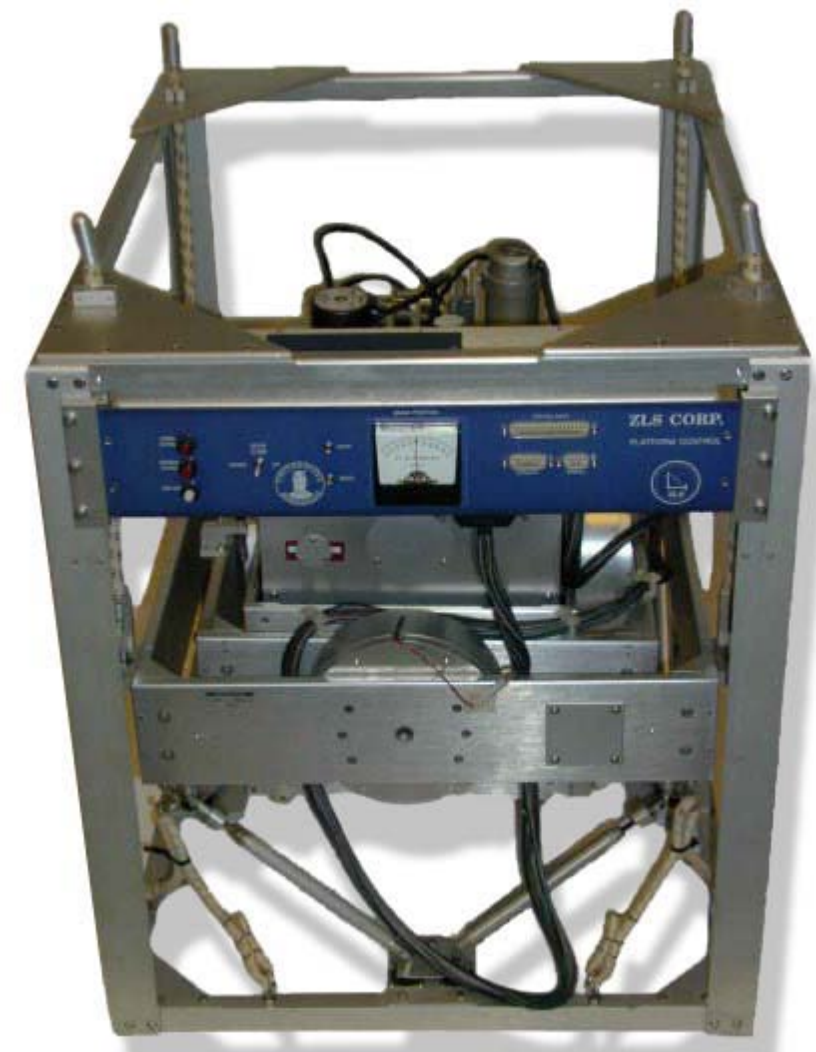
Example of a shipborne gravimeter: LC&R 5-meter
