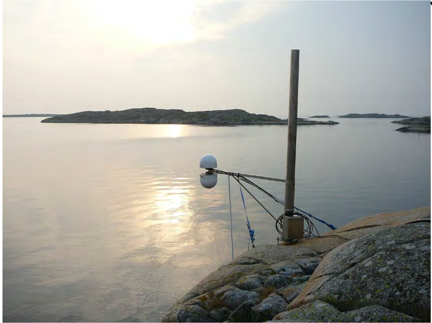
Bubbler and radar sensor tide gauge
