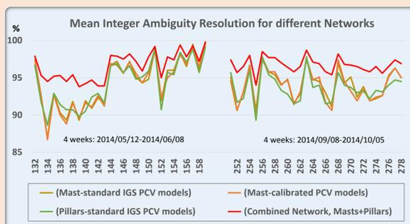
Figure 4: Mean wide-lane integer ambiguity resolution for the different networks.
