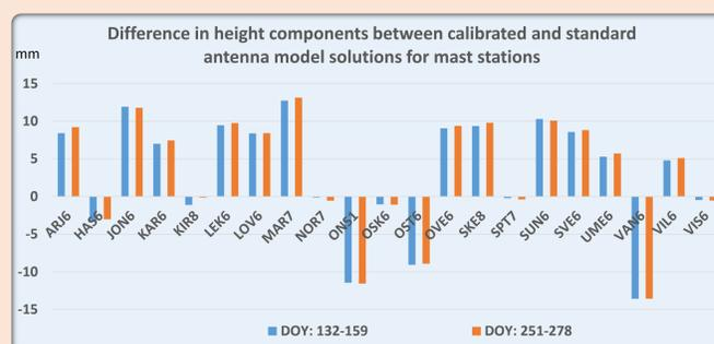
Figure 5: Difference in height components between individually calibrated and standard antenna model solutions for 21 mast stations. The blue and brown colors represent two independent combined solutions for two different seasons and look similar.
