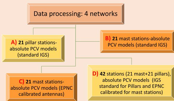
Figure 2. Overview of analyzed networks. Networks A, B and C with 21 stations had a total of 210 baselines. The combined network (D) with 42 stations had 861 baselines.
