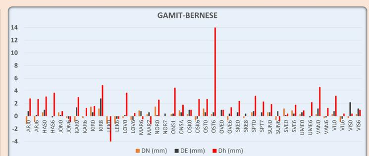
Figure 6: The difference between GAMIT and BERNESE (5.2) solutions in geodetic coordinates for 4 weeks data (140908-141005). Average differences in north, east and height coordinates are 0.1 mm, 0.5 mm and 1.8 mm respectively. Stations with relatively large height differences, such as OST6 and KIR8 should be further investigated.
