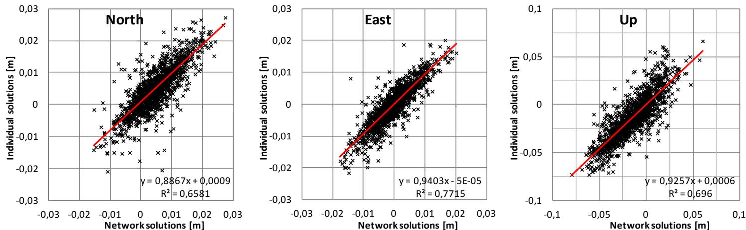
**Figure 6.** Correlation between network and individual solutions for North (left), East (middle) and up (right) components.
