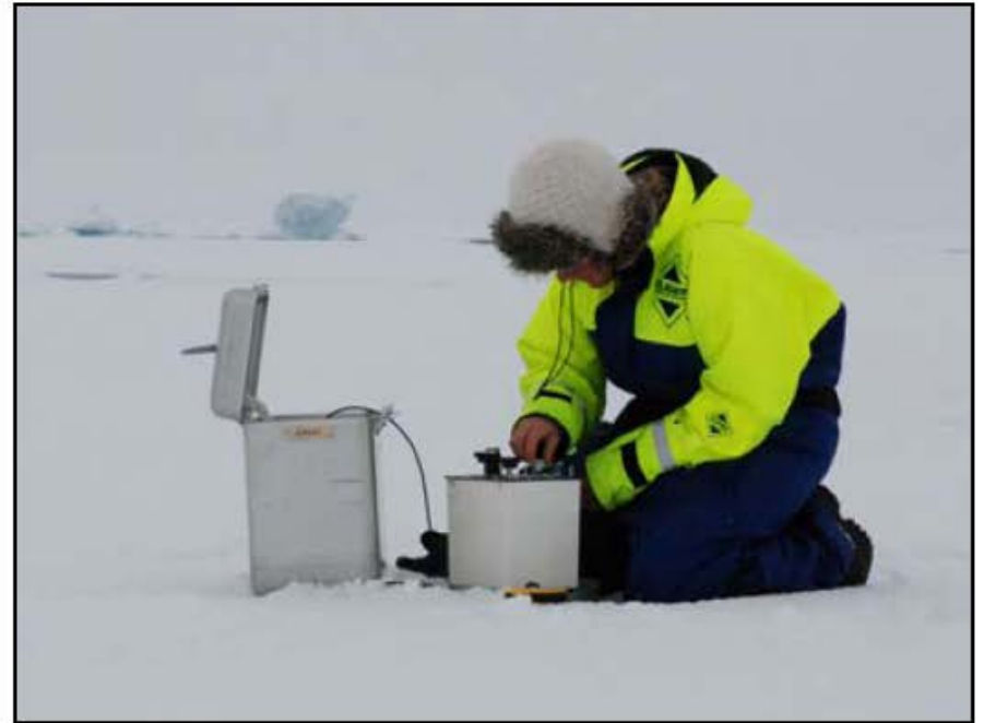
Figure 3 LaCoste and Romberg land gravimeter (left). Photo: Henriette Skourup. Gravity measurements on the sea ice (right). Photo: Adam Jeppesen.
