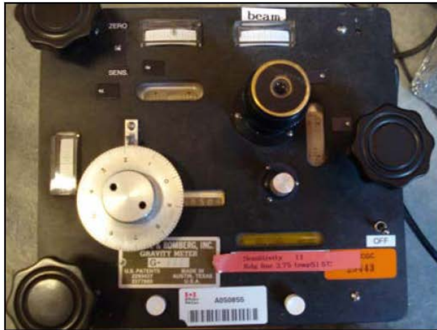
Figure 3 LaCoste and Romberg land gravimeter (left). Photo: Henriette Skourup. Gravity measurements on the sea ice (right). Photo: Adam Jeppesen.
